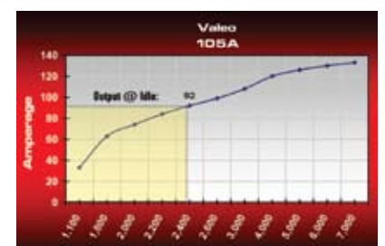
ALTERNATOR RPM (rotor speed) Alternator RPM is typically 3x engine speed; see FAQ's pg. 52
