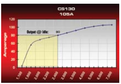
ALTERNATOR RPM (rotor speed) Alternator RPM is typically 3x engine speed; see FAQ's pg. 52
