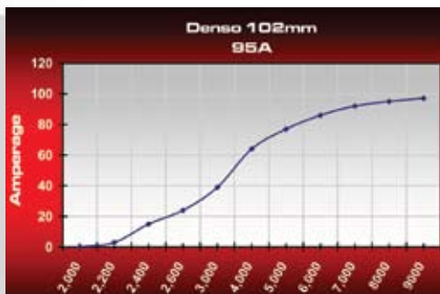
ALTERNATOR RPM (rotor speed) Alternator RPM is typically 3x engine speed; see FAQ's pg. 52
