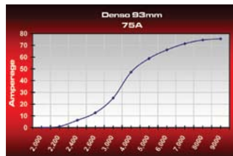
ALTERNATOR RPM (rotor speed) Alternator RPM is typically 3x engine speed; see FAQ's pg. 52
