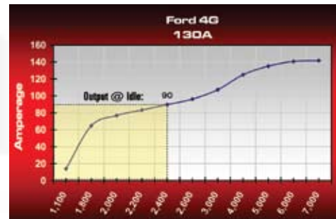
ALTERNATOR RPM (rotor speed) Alternator RPM is typically 3x engine speed; see FAQ's pg. 52
