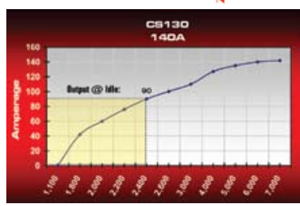
ALTERNATOR RPM (rotor speed) Alternator RPM is typically 3x engine speed; see FAQ's pg. 52
