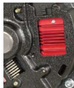
Close-up showing XS Volt regulator.
