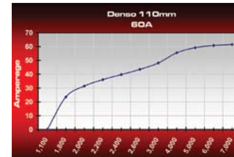
ALTERNATOR RPM (rotor speed) Alternator RPM is typically 3x engine speed; see FAQ's pg. 52
