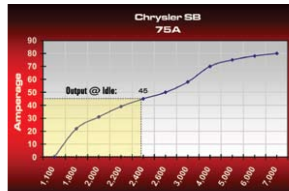
ALTERNATOR RPM (rotor speed) Alternator RPM is typically 3x engine speed; see FAQ's pg. 52
