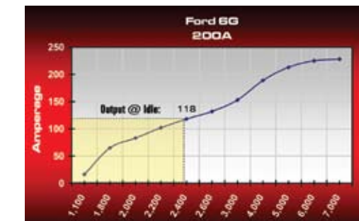
ALTERNATOR RPM (rotor speed) Alternator RPM is typically 3x engine speed; see FAQ's pg. 52
